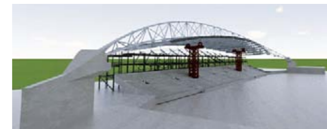
The East Stand's roof truss will be assembled in three sections and lifted onto temporary trestles which will remain in place until the opposite West Stand is completed
