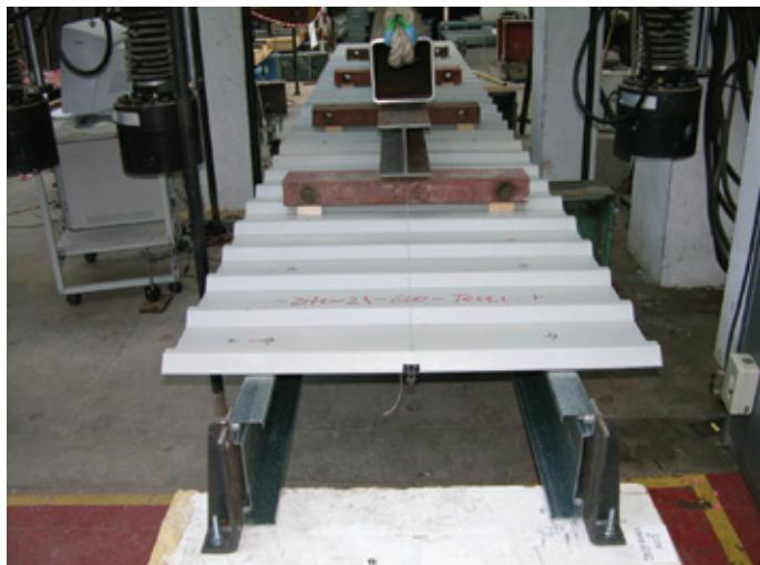
Load tests with cladding fixed to flanges
